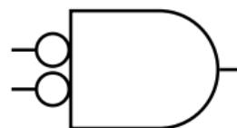
$$\overline{a \cdot b} = \overline{a} + \overline{b}$$
